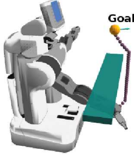
Fig. 7: This is an example when h_{endeff} is capable of guiding the search in a direction that is infeasible for a manipulator to follow. Shown in purple is the least-cost path suggested by h_{endeff} from the start configuration to the goal pose.
