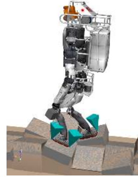
Fig. 1: Robot walking over uneven terrain course with friction cones (cyan)
