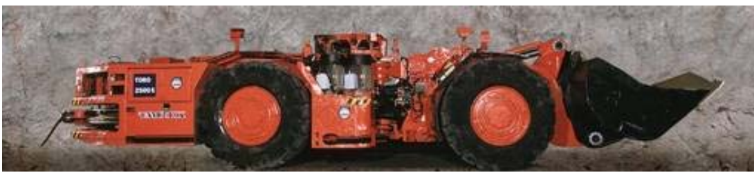
Fig. 2. Side view of the Tamrock Toro 2500 electrical wheel loader; length: 14 meters, operating weight: 76 tonnes, and capacity: 25 tonnes.
