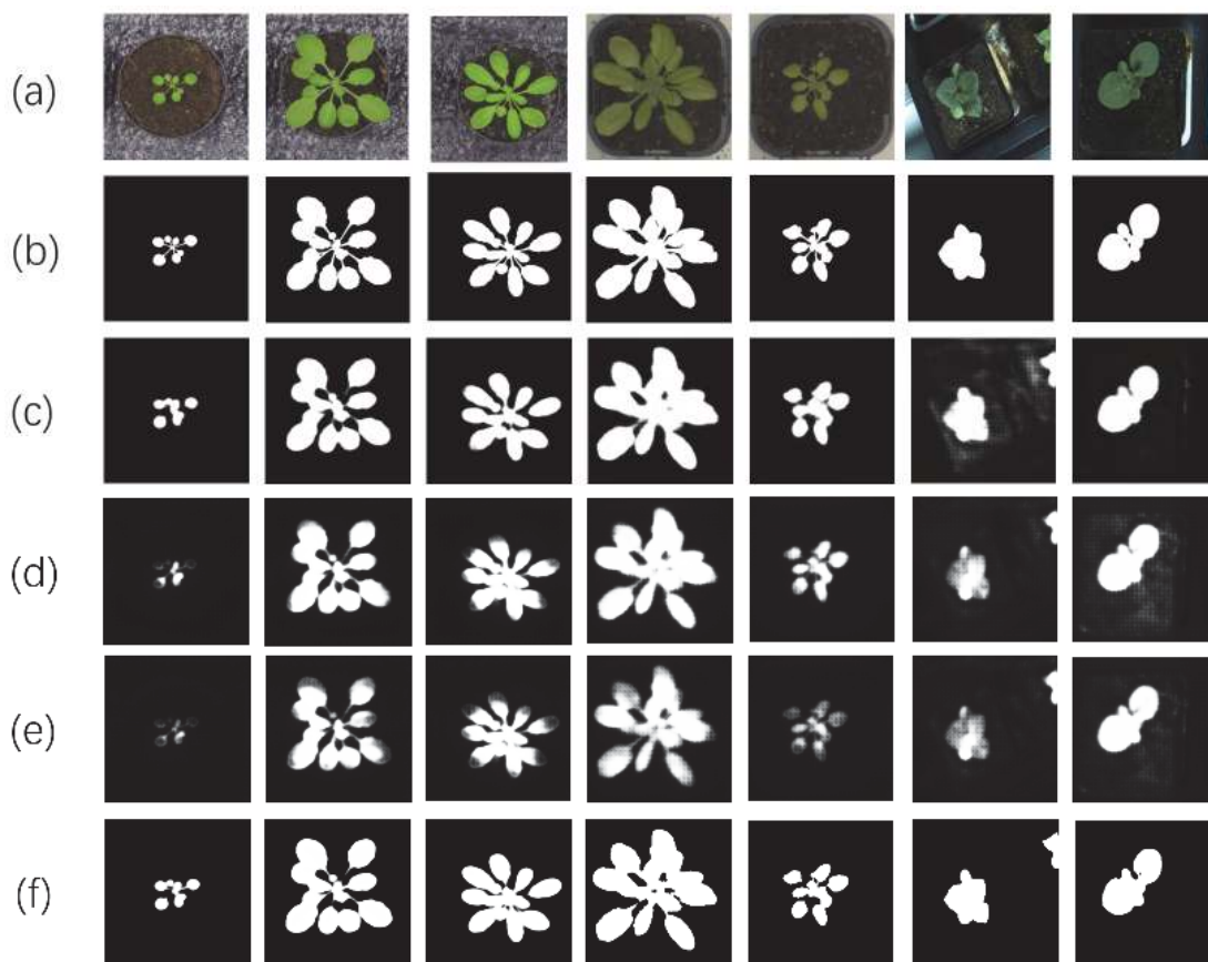
Figure 8. Segmentation results for different activation functions. (a) the original image in the test set; (b) the ground-truth; (c)-(f): the segmentation results of the models using (c) ReLu; (d) Sigmoid; (E) Tanh; (f) Leaky-ReLu.
