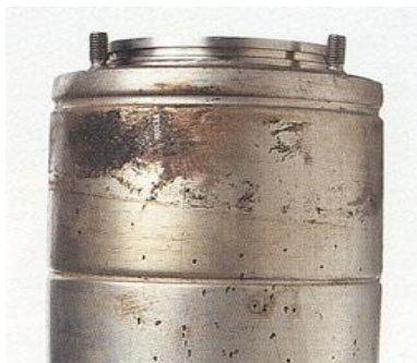
Figure 1: Pitting corrosion on a stainless-steel stator housing operating in seawater [29]
