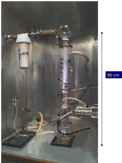
Figure 1. The plasma reactor for thin polymer film coating of the nanotubes.
