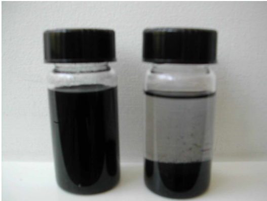
Figure 5. Solutions with coated (left) and uncoated (right) WMCNT's.
