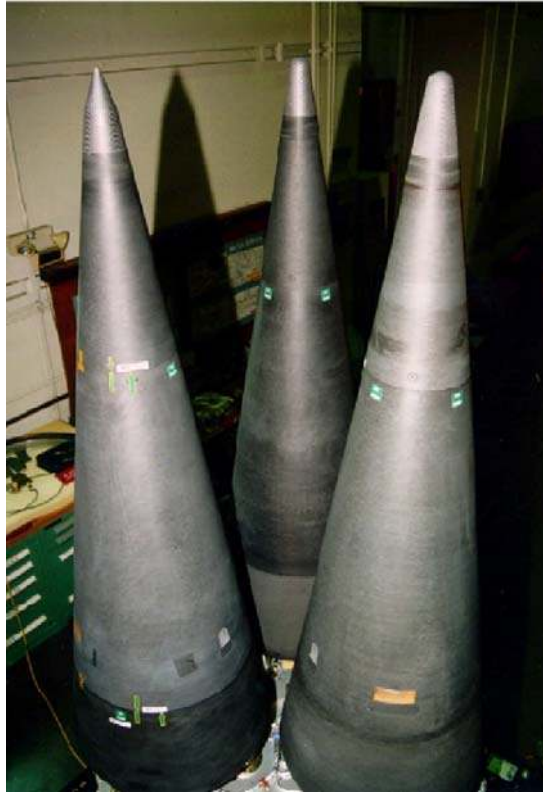
Figure 2: Dummy MIRV warheads on a Minuteman III Intercontinental Ballistic Missile (the left one has a modified sharp leading edge design as a part of the SHARP program at NASA Ames Research Center).
