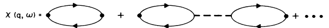
FIG. 1. Diagrams for density-density correlation function, to leading order in 1/N . The heavy dots denote density vertices. The solid lines with arrows represent electron Green's functions obtained from the inverse of L_F , Eq. (2a) in the text. The dashed line represents either bare boson propagators obtained from inverting L_B , Eq. (2b) in the text, or the Coulomb interaction 4\pi e^2 / q^2 N . The vertices at which boson or Coulomb lines join fermion lines are obtained from L_I , Eq. (2c) and L_c , Eq. (2d), respectively.
