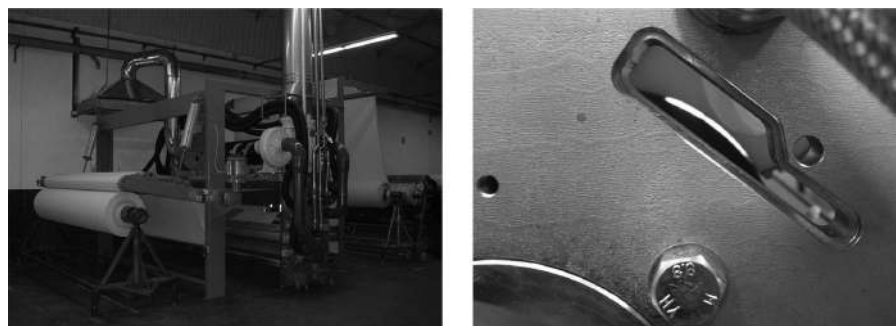
Figure 2. Industrial air DBD plasma apparatus (left) and detail (right) of the plasma discharge (white halo in the centre) for cotton pre-treatment in a Portuguese textile company.
