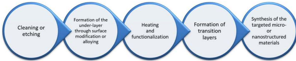
FIG. 3. Typical process workflow for the assembly of nanostructured surface architectures. Starting from surface cleaning or removal of upper damaged layers, several sub-layers are formed by deposition and further, the targeted structured material is formed upon functionalization of the deposited layers.
