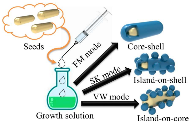
Figure 3. Schematic illustration of three different growth modes of plasmonic heteromers using seed-mediated approaches.
