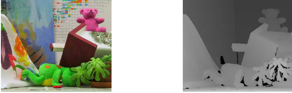
Figure 1. Example texture image (left) and the corresponding depth map (right). 2 A typical depth image contains regions of linear depth changes bounded by sharp discontinuities.
