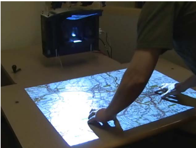
Figure 11: Flow field-based manipulation of objects applied to panning, rotating, and zooming a high resolution map.
