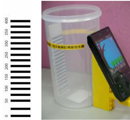
Figure 3. Pattern bars are shown on the right. The pattern bars painted on the outer surfaces of water bottle are shown on the left.
