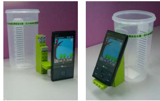
Figure 1. Three physical components of the Playful Bottle prototype: (a) water bottle, (b) bottle-phone attachment made from LEGO bricks, (c) a mobile phone, and (d) the mobile phone clipped to the bottle through the LEGO attachment.
