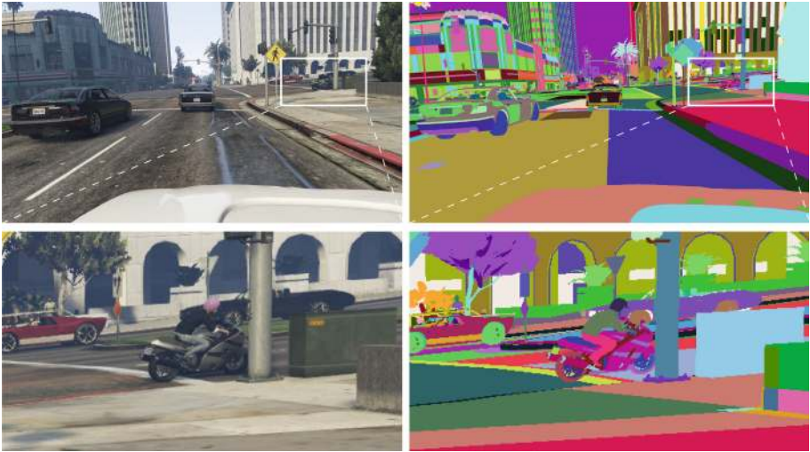
Fig. 2. Illustration of the patches used as atomic units during the annotation process. Top left: one of the images in our dataset. Top right: patches constructed by grouping pixels that share a common MTS combination. Different patches are filled with different colors for illustration. Bottom row: partial magnifications of the top images. (Color figure online)
