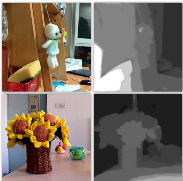
Fig. 6. Examples of soft layer mask extraction. Left: the central view of the light field. Right: the estimated depth map.
