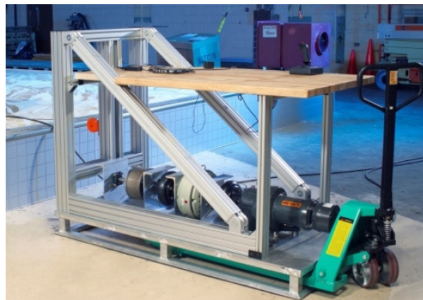
Figure 13: Drawbar pull rig with adjustable load at the SLOPE facility[26].
