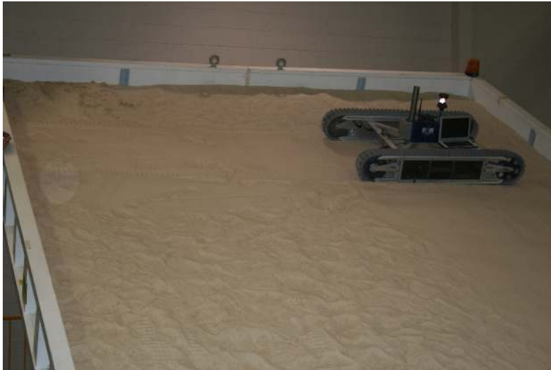
Figure 16: Cross Slope test at 30 degrees.
