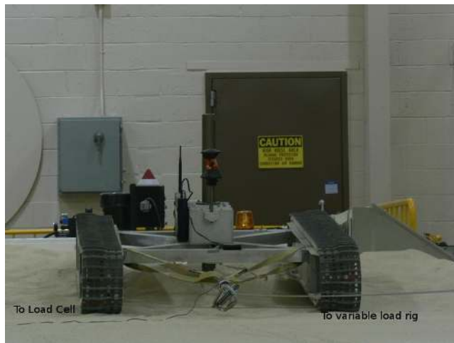
Figure 15: Draw bar pull test setup with lines going to a load cell and the variable load source.
