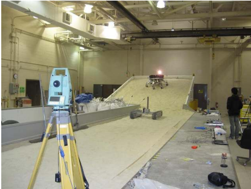
Figure 12: Test setup with surveying instrument (on the left) and prism (bright spot) mounted on a rover at NASA GRC SLOPE facility.
