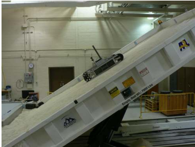
Figure 14: Descent test at 31 degrees.
