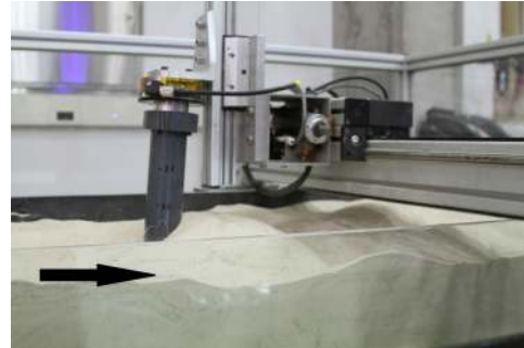
Figure 29: Bulldozing at end of 2 inch diameter plow. Black arrow shows direction of plow motion.
