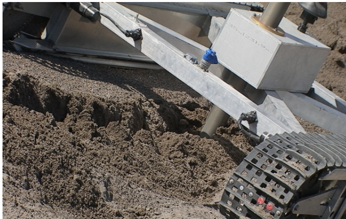
Figure 3: Icebreaker actuated plow. The box contains the motor and pinion for driving the plow into the ground [28].
