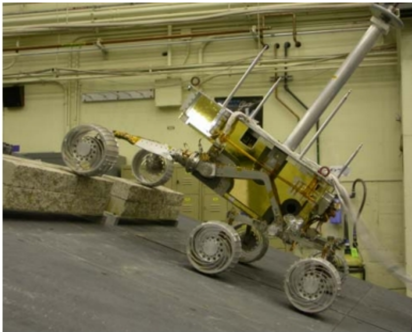
Figure 22: MER test model on a 20 degree slope navigating over 25cm obstacles[2].
