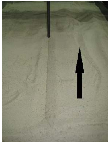
Figure 26: Shape of path created by 0.5 inch diameter plow. Black arrow shows direction of plow motion.
