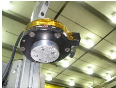
Figure 25: Six axis ATI Delta Transducer load cell used for the wheel test-bed.
