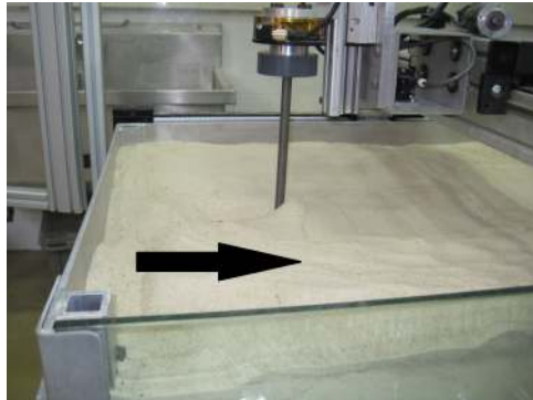
Figure 28: Bulldozing at end of 0.5 inch diameter plow. Black arrow shows direction of plow motion.
