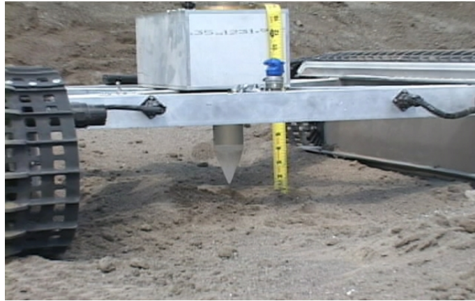
Figure 4: Icebreaker actuated plow. Conical lexan tip is used to penetrate into the ground [28].
