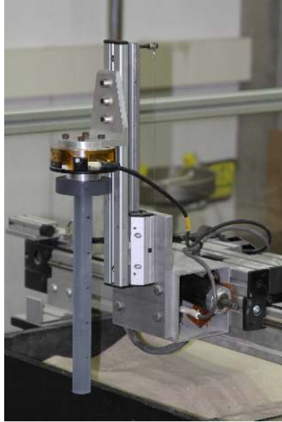
Figure 24: Closeup of test-bed mechanism with 1 inch plow attached.
