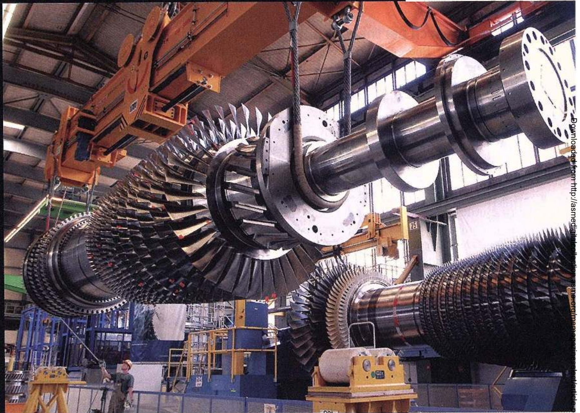
▲ Technicians prepare the Siemens Energy SGT5-8000H for delivery to a power plant in Irsching, Bavaria. The turbine weighs 440 metric tons.
