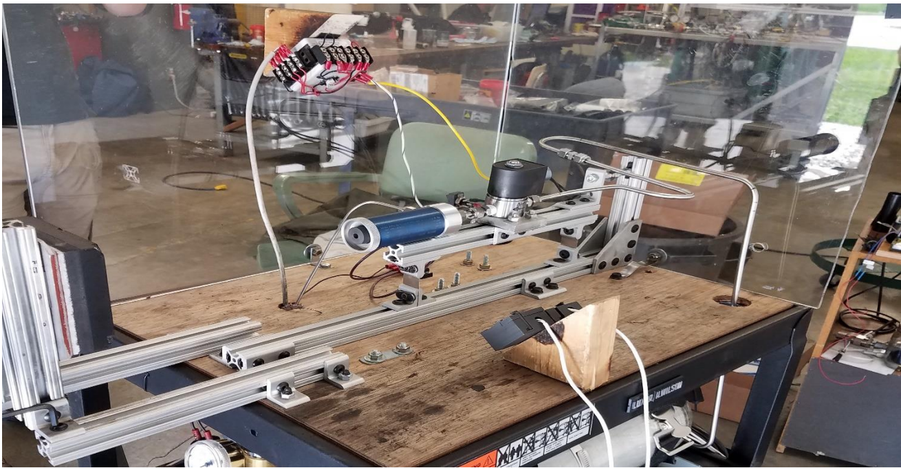
Fig. 11 25-N Thruster Mounted on Demo Test Rig stand with LED and Photometers installed.
