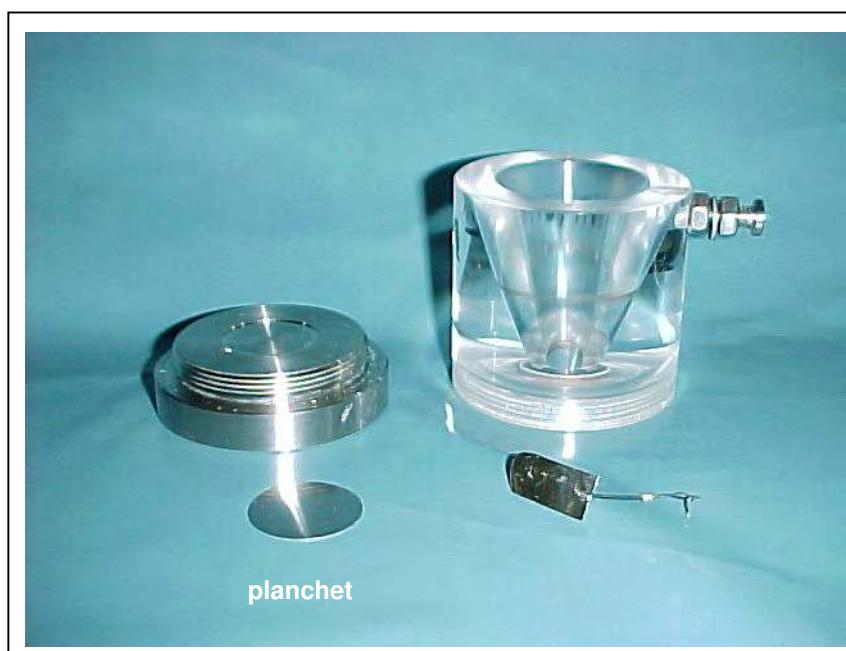
Figure 2.4.2 The main constituents of the electrodeposition cell. The planchet where the sample is electrodeposited is also shown.
