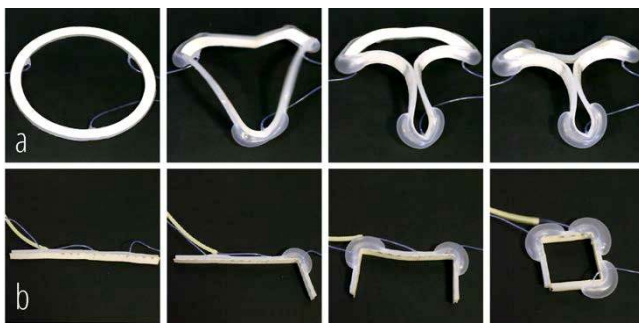
Figure 7: Specifically designed crease patterns and respective control of airbags enabling dynamic transformation of shapes.
