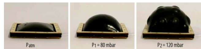
Figure 13: As the increase of air pressure, the surface deform from global to local region.
