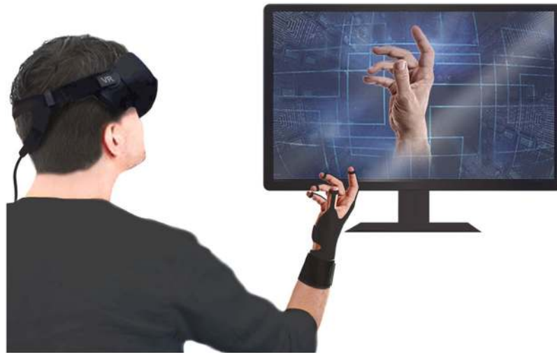
Figure 1. A glove for user interaction with VR. The glove transmits the hand motion of the user to the VR and transmits the stimulus to the user. The figures were created by the authors.
