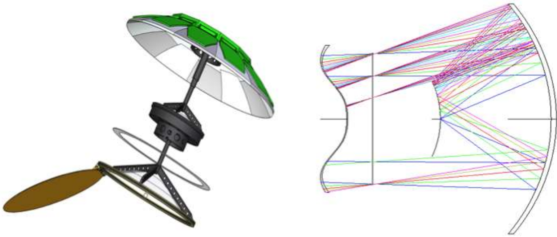
Figure 2: POEMMA mirrors: Right - optical design for a f/0.77 Schmidt mirror and corrector lens, with 45^\circ field of view (FoV); Left - POEMMA mirror and focal surface and shutter deployed.
