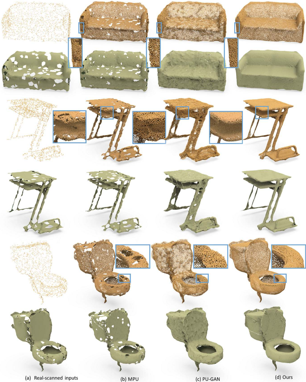
Figure 7. Comparing point set upsampling ( 16\times ) results and reconstructed 3D meshes using different methods (b-d) from real-scanned sparse inputs (a), while the bottom row shows the reconstructed meshes. Clearly, our method outperforms others on the local uniformity, contributing a better surface reconstruction.
