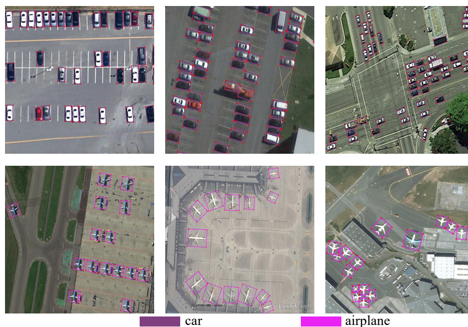
Figure 10. Visualization of the detection results of Point RCNN for the UCAS-AOD test set. The score threshold was set to 0.01. The red points and colored OBBs are the predicted corner points and the converted OBBs of PointReg.
