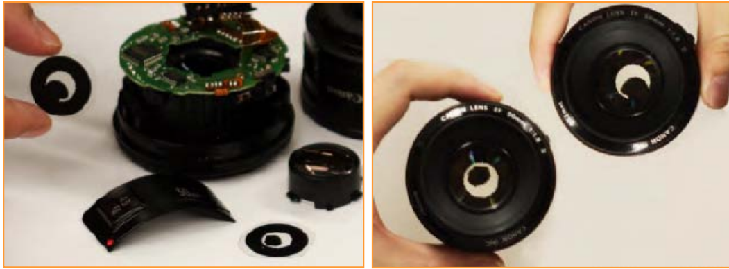
(a) A disassembled Canon EF 50mm f/2.8 lens (b) Two lenses with the optimized patterns inserted
