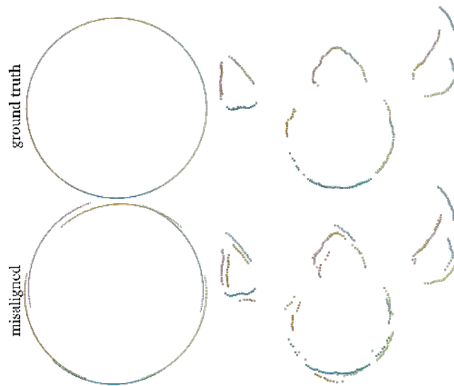
Figure 15: Cross section of cylinder (left) and armadillo (right) misaligned scans with \theta = 2^\circ . Each color corresponds to a scan from a single angle.
