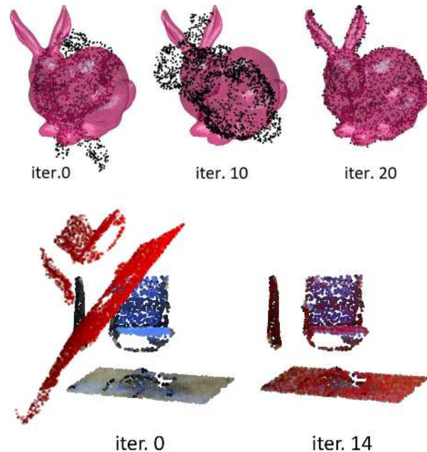
Figure 1: Point cloud registration of (Top) Stanford bunny [39] and (Bottom) raw indoor scan from S3DIS [1] with PointNetLK . Refer to Sec. 4.2 and Sec. 4.4 for more details. As the iterations progress, PointNetLK is able to successfully register the source points to the template model, even though it was not trained on these shapes. We include Bunny surface rendering for the sake of visualization.
