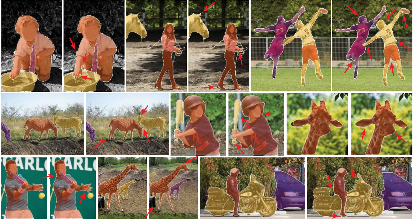
Figure 2: Example result pairs from Mask R-CNN [17] with its standard mask head (left image) vs. with PointRend (right image), using ResNet-50 [18] with FPN [25]. Note how PointRend predicts masks with substantially finer detail around object boundaries.
