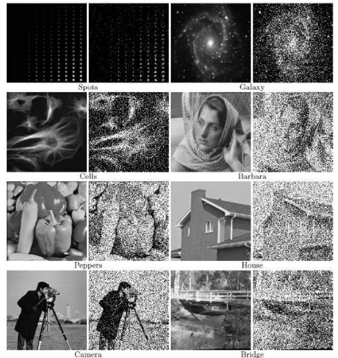
Fig. 3: No-noise images used in this article and synthetic Poisson-noise images with Peak = 2 ("Spots", "Galaxy", "Cells", "Barbara", "Peppers", "House", "Camera", "Bridge").
