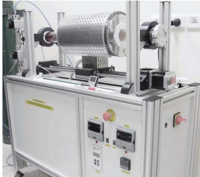
Figure 3.29: Custom built preform consolidator system.
