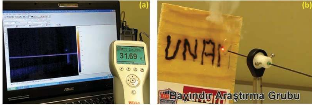
Figure 4.6: Heat profile of fiber during transmission of 40 W laser beam (with 32 W output power) (a) and burning of a wooden piece by output laser beam (b).
