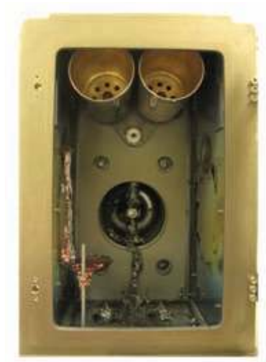
Figure 3.24: Picture of upgraded Elif evaporator system.
