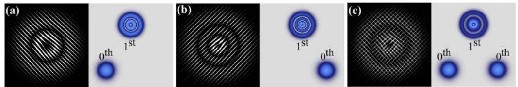
Figure 6. Schematic representation of the multiplexing principle. Binary hologram to generate the modes (a) LG_1^2 and (b) LG_2^{-1} , (left panel). The frequency value of each linear phase is properly chosen to shift the beam to the desired position, as shown on the right panel of (a,b). An example of a multiplexed hologram composed of the holograms shown on (a,b) is shown on the left panel of (c), whereas the overlapping of both first diffraction orders is shown on the right panel. Here, for the sake of clarity we only show the first and zero diffraction order, higher diffraction orders were omitted.
