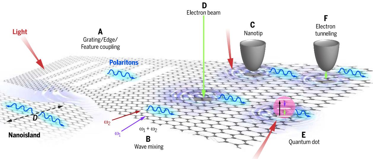
**Fig. 2. Launching and visualizing polaritons.** (A to F) Excitation and probing of vdW polaritons (blue arrows) can be achieved using (A) periodic structures (110–112), (B) nonlinear wave mixing (95), (C) antenna-like nanotips (20, 21), (D) electron beams (113), (E) quantum dots and localized emitters (114, 115), and (F) electron tunneling (116). Polaritons produced by processes shown in (A) to (C) maintain phase coherence with respect to the external
