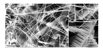
FIG. 72. SEM image of nanocombs consisting of nanoribbons grown along the  $[2\bar{1}\bar{1}0]$  direction with  $\pm(0001)$  side surfaces, on which NWs are more slowly formed along the [0001] direction, while no growth occurs along the  $[000\bar{1}]$  direction. Reprinted with permission from Wang *et al.*, Phys. Rev. Lett. **91**, 185502 (2003). Copyright 2003 American Physical Society.
