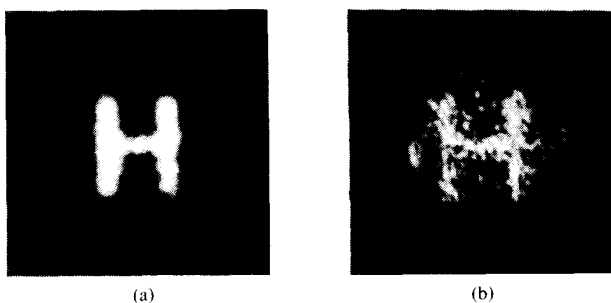
Fig. 10. Photographs of the x -polarized phase-conjugate images of the letter H for (a) (\phi/\phi_0)^2 = 0.015 and (b) (\phi/\phi_0)^2 = 0.74 .
