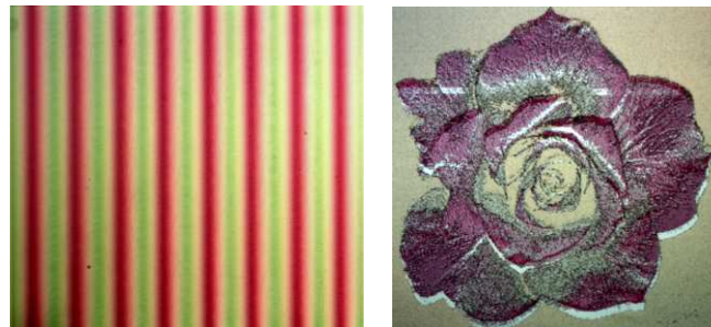
Fig. 3. (Left) Coloration of birefringent structure in crossed polarizers when additional constant retarder is added. (Right) Birefringent rose written in silica glass with femtosecond laser in 1 mm \times 1 mm square.
