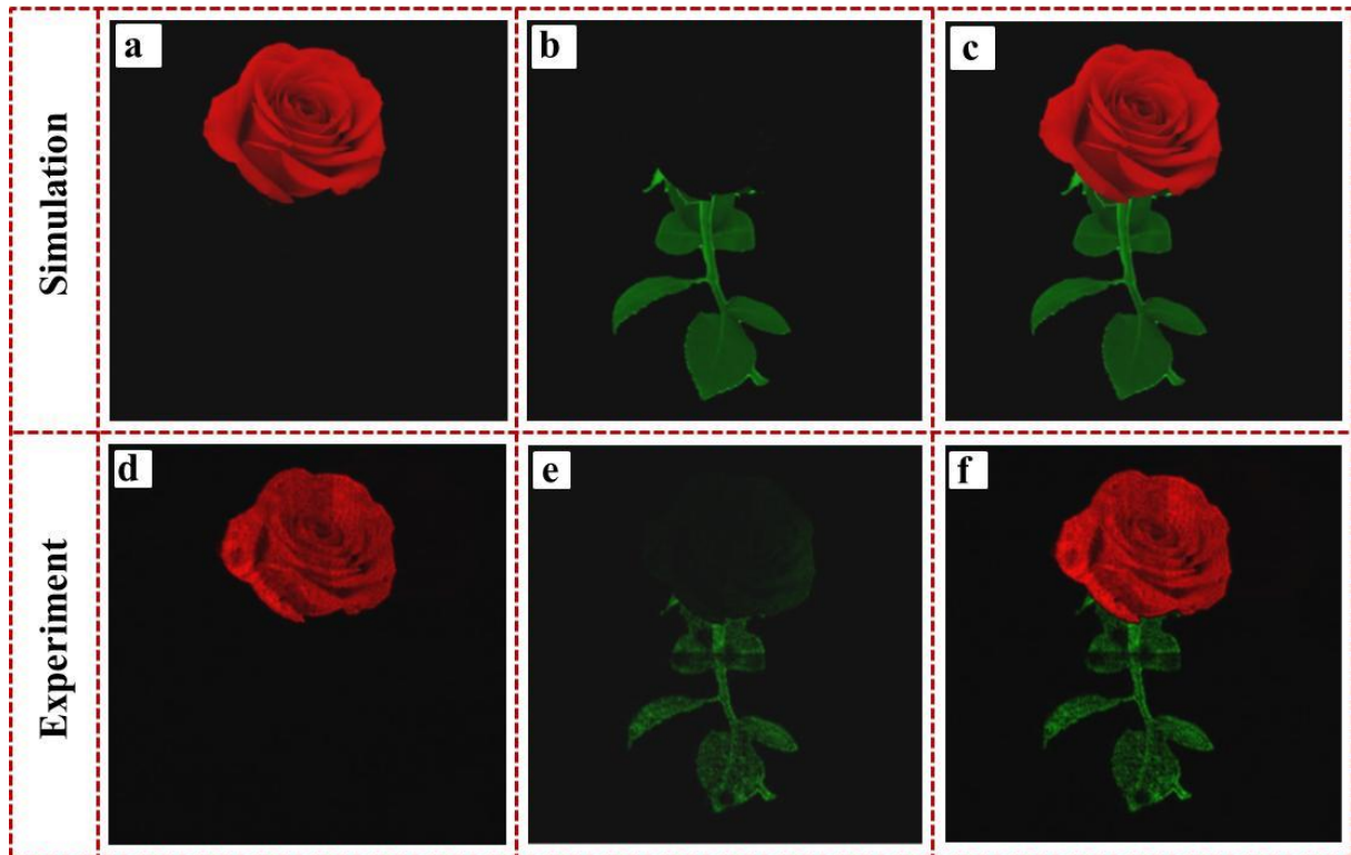
Fig. 3. Simulated and experimental results of the polarization encoded color image. The revealed color image when illuminated with light at the wavelengths (a) and (d) \lambda=660 nm; (b) and (e) \lambda=550 nm; (c) and (f) \lambda=660 nm and 550 nm. The images in the first row and second row represent the simulated and experimental results, respectively.
