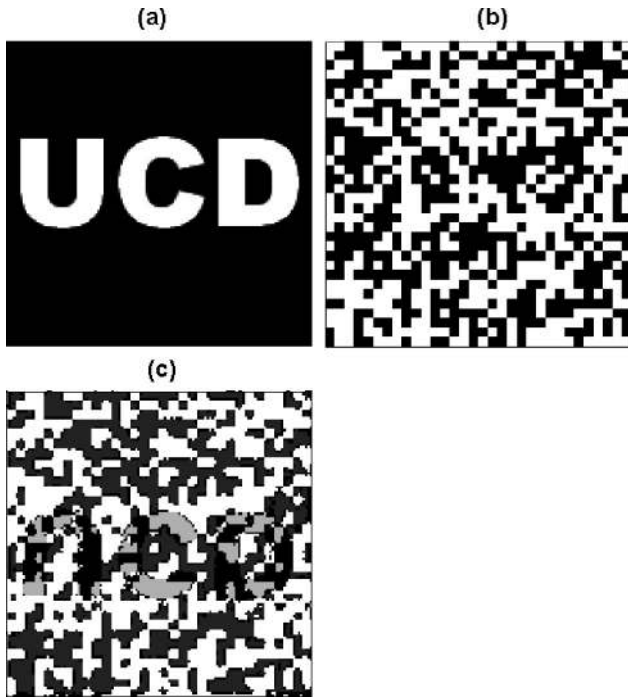
Fig. 9. (a) and (b) Two input signals. (c) Multiplexed output signal from the optical system. Each gray level in (c) represents a polarization state.
