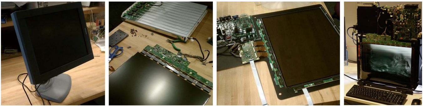
Figure 5: Constructing the polarization field display prototype. Four monochromatic LCDs were modified to create a single multi-layer LCD. Photographs depict from left to right: an unmodified Barco E-2320 PA LCD, the liquid crystal panel and backlight after removing the case and power supply, a modified panel mounted on an aluminum frame, and the assembled prototype.
