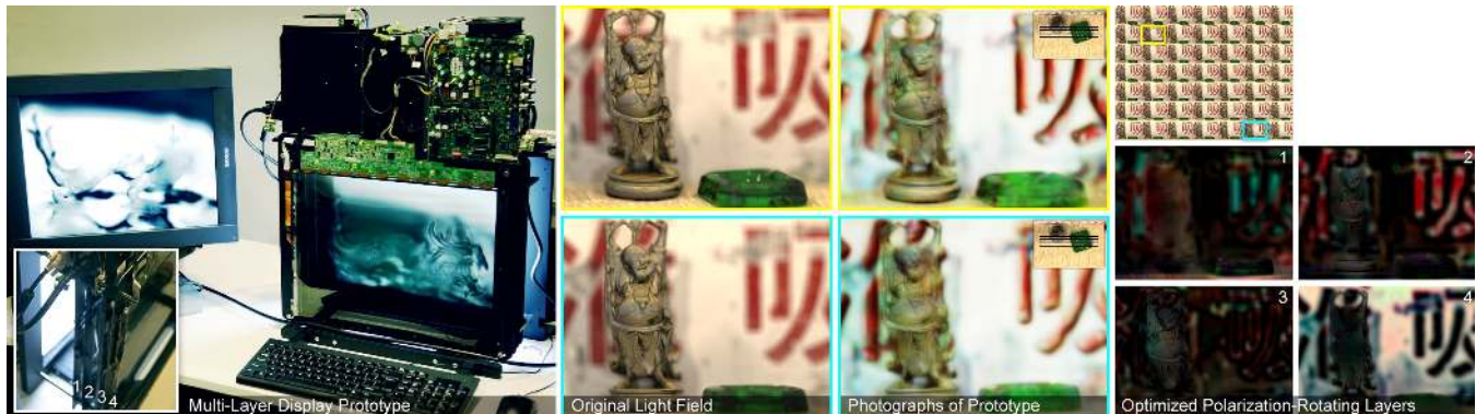
Figure 1: Dynamic light field display using polarization field synthesis with multi-layered LCDs. (Left) We construct an optically-efficient polarization field display by covering a stack of liquid crystal panels with crossed linear polarizers. Each layer functions as a polarization rotator, rather than as a conventional optical attenuator. (Right, Top) A target light field. (Right, Bottom) Light fields are displayed, at interactive refresh rates, by tomographically solving for the optimal rotations to be applied at each layer. (Middle) A pair of simulated views is compared to corresponding photographs of the prototype on the left and right, respectively. Inset regions denote the relative position with respect to the display layers, shown as black lines, demonstrating objects can extend beyond the display surface.
