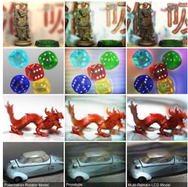
Figure 6: Polarization field display using the multi-layer prototype. The central views for the “Buddha”, “dice”, “dragon”, and “car” scenes are shown. Views predicted by the polarization rotator model (Equation 5) and the multi-domain LCD model (Equation 15) are compared in the left and right columns, respectively. Photographs of the prototype are shown in the middle. Section 4.2 and Appendix A quantitatively assess performance and artifacts.
