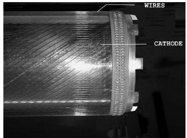
Fig. 3. Detailed view of the tip of the internal cylindrical chamber showing the helicoidal strips and the wires. The pitch angle of the strips is 34^\circ .
