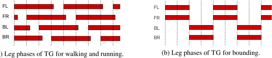
Figure 6: Leg phases for 2 different gaits used for TG. For each leg, the red bar indicates the duration of the stance (compared to swing represented by empty areas). FL: Front Left, FR: Front Right, BL: Back Left, BR: Back Right.
