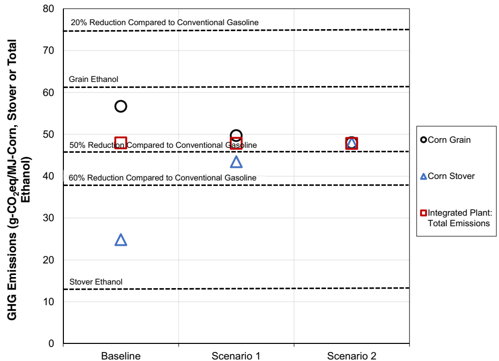
Fig. 5 Net GHG emissions for corn grain and stover ethanol for the baseline and the two alternative CHP usage scenarios. The 20, 50, and 60 % GHG reduction lines represent the targets for the corresponding reduction in GHG emissions compared with gasoline at 94 g-CO 2 eq/MJ. The lines for grain ethanol and stover ethanol represent the GHG emissions to produce ethanol in a non-integrated scenario
