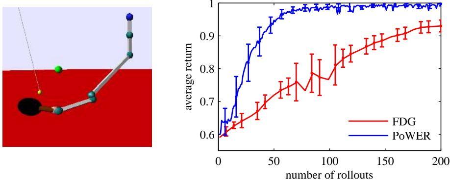
(a) The tasks consists of striking the yellow ball hanging on an elastic string such that it hits the green target.
