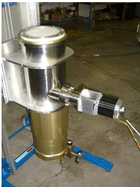
Figure 5. Left: Fully assembled POLOCAM test cryostat with warm motor and ferro-fluidic feedthrough assembly. Right: FTS frequency response of the POLOCAM cryostat (black). The polarization efficiencies (red) and cross-polarization leak (blue) data of unit-level testing of the waveplate from Figure 2 are also shown for reference.
