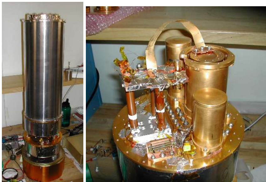
Figure 4. Left: Cryostat with 4 K POLOCAM radiation shield. Right: Interior view of the cryostat, showing the 4 K stage, fridge, ultracold stage, and bolometer/feedhorn assembly.
