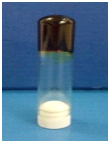
Fig. 1. The view of a gel electrolyte based on PVA.
