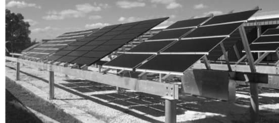
Figure 5: Hot and humid testing of thin-film modules at FSEC, Cocoa, Florida
