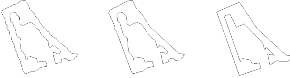
Fig. 2. (a) \rightarrow (b): noise elimination. (b) \rightarrow (c): extraction of relevant line segments.
