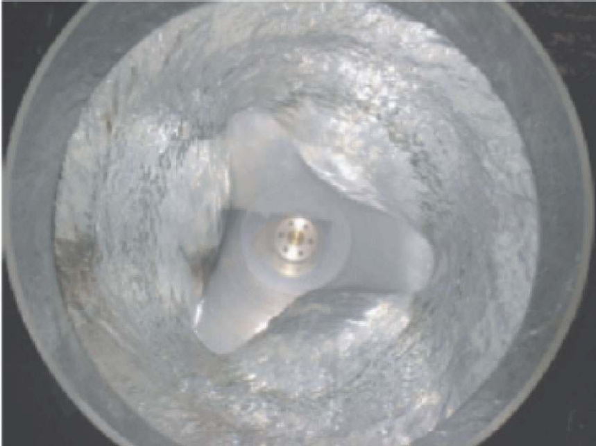
FIGURE 2. Dry triangle with H = 4 cm and f = 2.4 Hz. Inside the faint circle the bottom plate is dry. Between the faint circle and the rotating polygonal contour there is a thin fluid layer.
