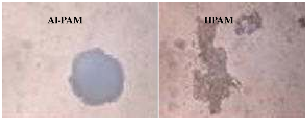
Figure 6-1-7 Morphology of the floccules formed from kaolin suspensions by Al-PAM and HPAM [4]
