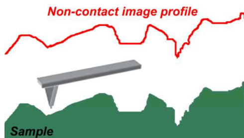
Figure 4. Schematical depiction of the non-contact AFM mode.
